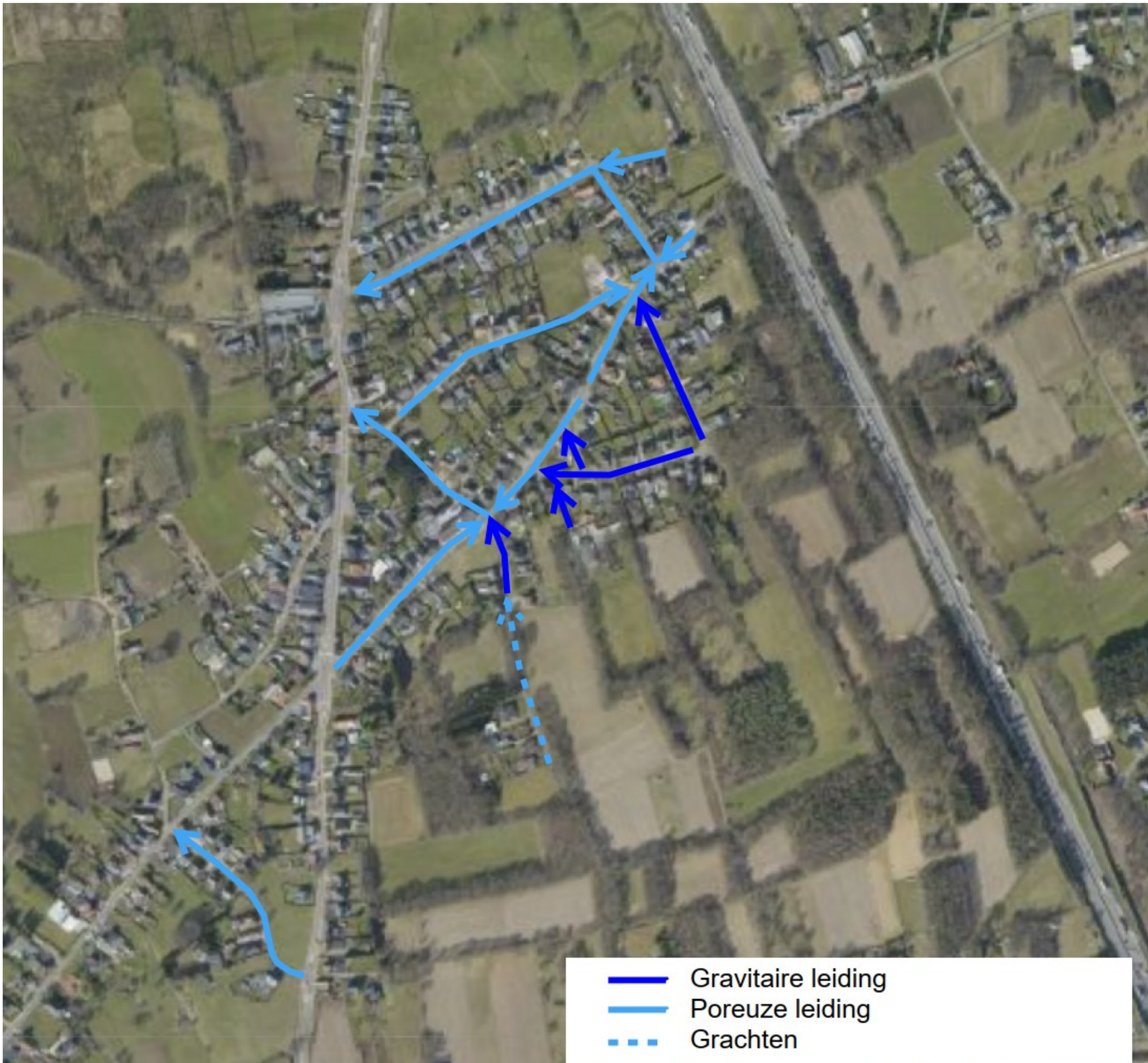
Schema afwatering hemelwater
